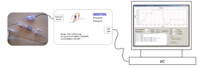
The sensor is a standard bridge type of sensor used for IBP measurements ( $5\mu V/V/mmHg$ ). The USB module contains special circuitry to ensure high accuracy measurements can be derived from such a sensor, and is combined with non-linear compensation in the PC software.
